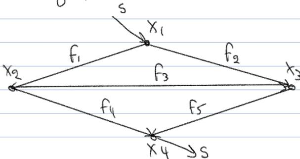
We can associate an incidence matrix  $A$  with this graph. Each row corresponds to a node, and each column to an edge, with
