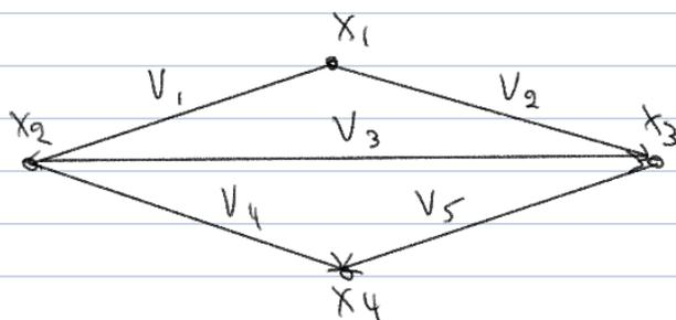
Solving  $A^T \underline{x} = \underline{v}$  tells us what potentials we need to put on the nodes to achieve the desired voltages. For example, the first row of  $A^T \underline{x} = \underline{v}$  reads  $-x_1 + x_2 = v_1$ . This is **Kirchoff's voltage law!**
